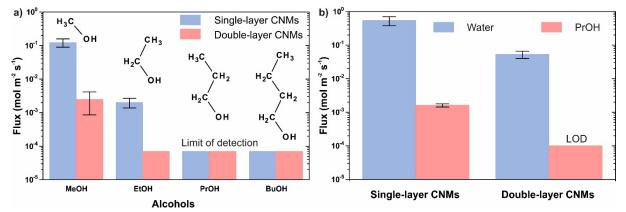
Figure 2. a) Transmembrane flux of pure alcohols in single- and double layer CNMs under saturation vapor pressure [3]. b) Transmembrane flux of  $D_2O$  and  $C_3H_7OH$  in single- and double layer CNMs upon exposure to the azeotropic mixture [3].
