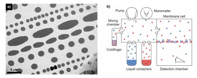
Figure 1. a) Helium ion micrograph of a large area TPC CNM suspended over a TEM grid [1]. b) Schematic of the ACP measurements with vaporous mixtures [2].
